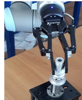
Figure 4. UR10 manipulator robot with 2F-140 adaptive gripper
